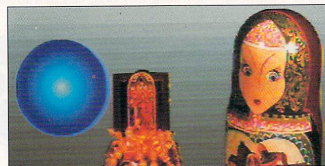
A 600x400 24-bit test image (top, 371K) is followed by 16-color (93K) and 256-color (196K) versions that show color banding and dithering. Next down, the 169K HAM8 rendition looks almost as good as the original. The three-bitplane DCTV image (bottom, 56K) shows banding and artifacting, though less pronounced in NTSC.
